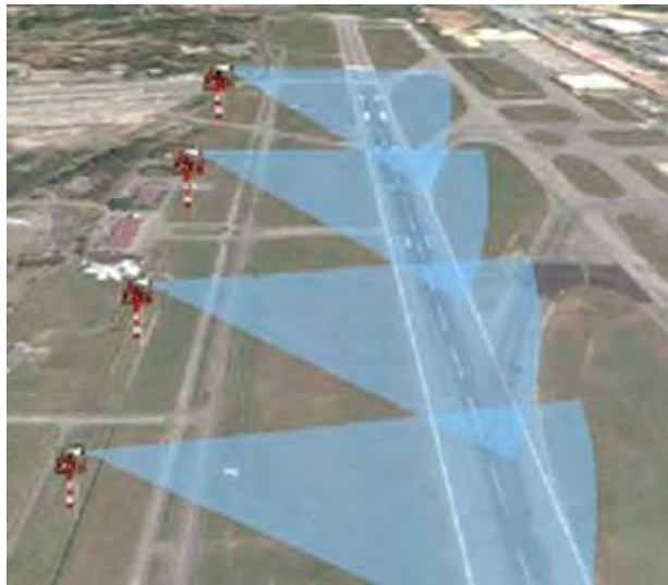
Figure 2. Typical iFerret Installation Illustrating how Multiple Sensors Operate to Provide Surveillance Along the Length of a Runway
