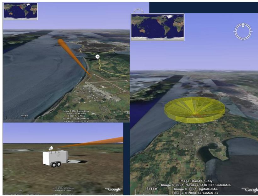
Figure 7. Representations of Dish Antenna Coverage as a Single Cone (Left) and the Full Volume Covered as the Dish Rotates (Right)
