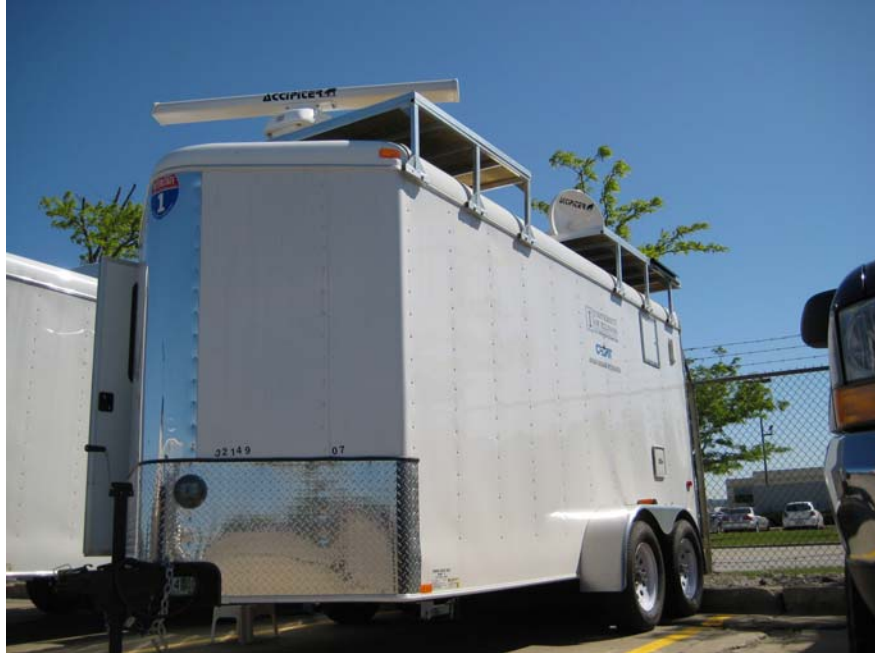
Figure 18. Slotted Array and Parabolic Dish Antennae Installed on a CEAT Trailer
