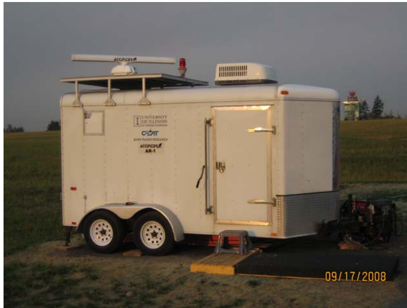
Figure 4. Slotted Array Antenna on CEAT Trailer Located at SEA
