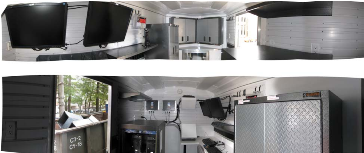
Figure 19. Panoramic Views of the Interior of a CEAT Radar Trailer Equipped With an Accipiter® AR2 System With Two Radars
