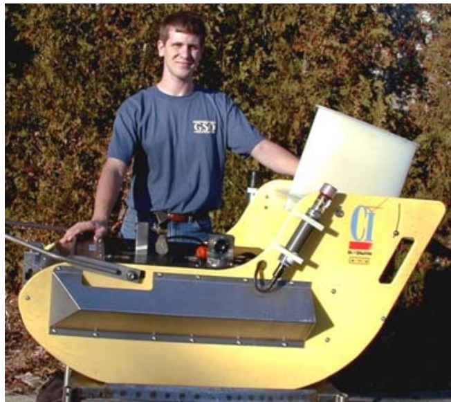
Figure 2A. Northeast Fisheries Science Center Systematic measurements are made of the LME by using towed bodies such as the Mariner Shuttle, depicted here (Lord 1998).
