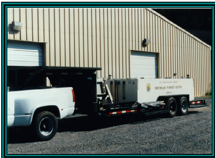
Figure 5.- Trailer-mounted sturgeon transport/holding tank with fold-down steps
