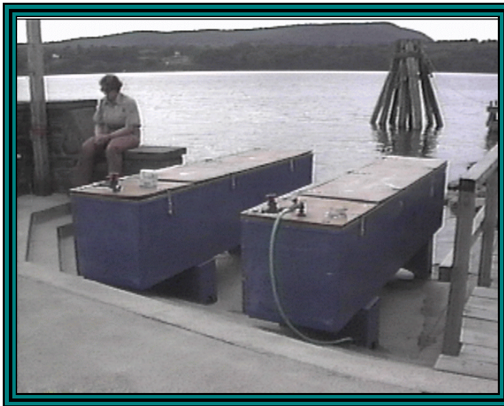
Figure 4.- Docksider sturgeon holding tanks with flow-through water supply
