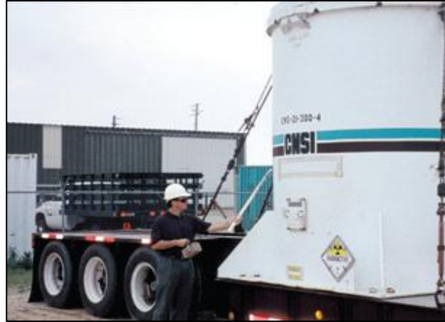
Figure 3 Type A Shipping Cask on Flatbed Trailer Source: SC DHEC, 2007
