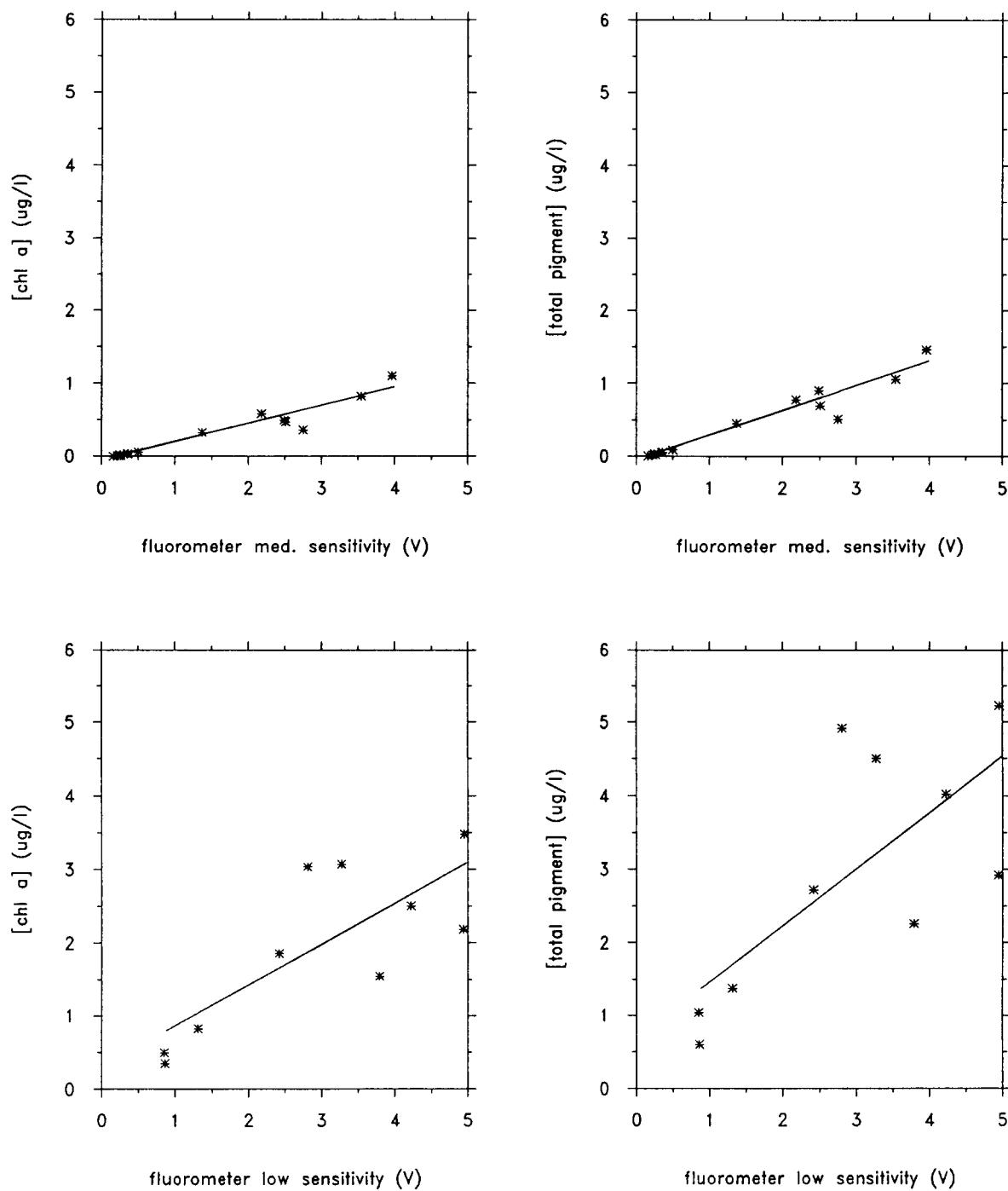
Figure 3. Plots of chlorophyll concentrations, pigment concentrations, and fluorometer measurements showing regression lines.
