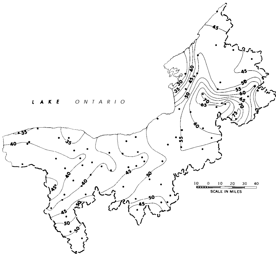
Figure 2. Isohyetal map of overland precipitation for the Lake Ontario Basin for 1972, in inches.
