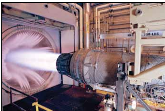
The F100 Engine for the F-15 and F-16 being Tested in SL-2
