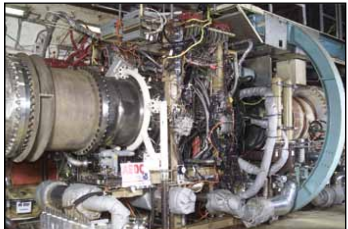
The Advanced Turbine Engine Gas Generator (ATEGG) Installed in J-1 for Core Testing
