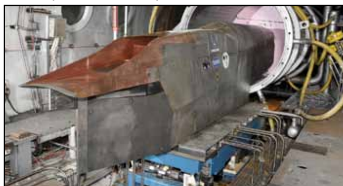
DARPA FaCET Test Article Installation
