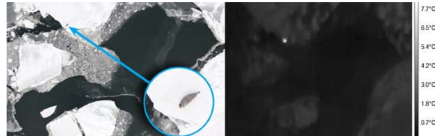
Figure 6. Paired thermal and visual images of a bearded seal on Bering Sea pack ice, collected during the 2012 survey. The images were collected using a Canon Mark III 1Ds digital SLR camera with a 100-mm Zeiss lens and an FLIR SC645 thermal imager mounted in the belly port of a fixed-wing aircraft flying at an altitude of 1,000 feet.
