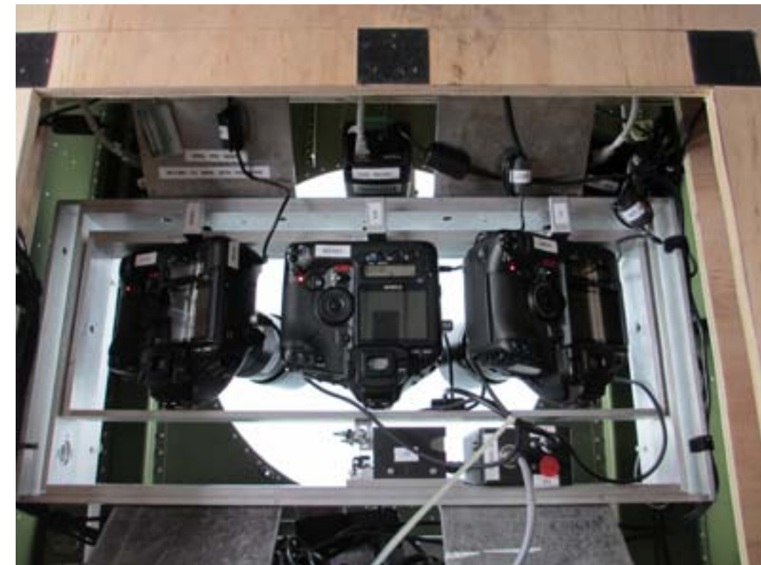
Figure 5. Paired Canon Mark III 1Ds digital SLR cameras and FLIR SC645 thermal imagers mounted in the belly port of a NOAA Twin Otter (N56RF) aircraft.
