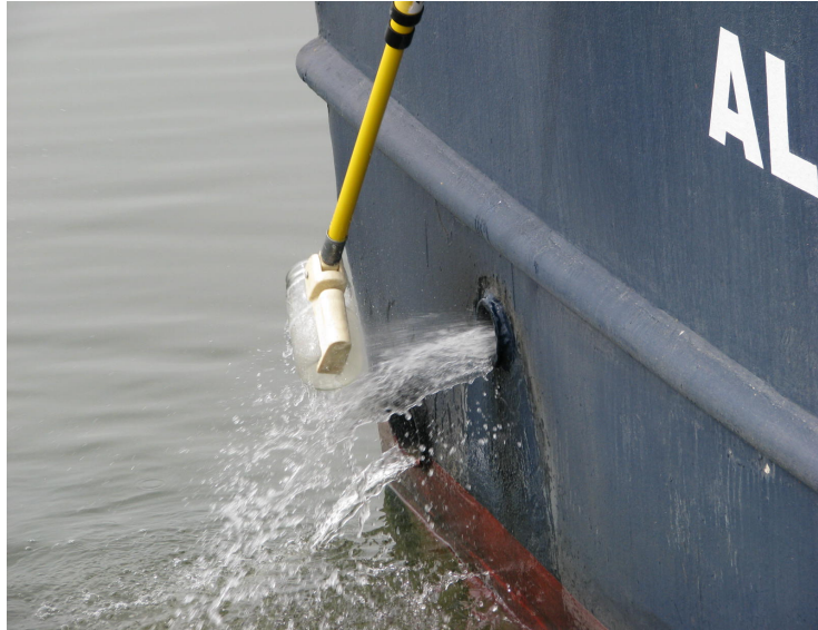
Collecting the Engine Effluent of a Water Taxi at Idle
