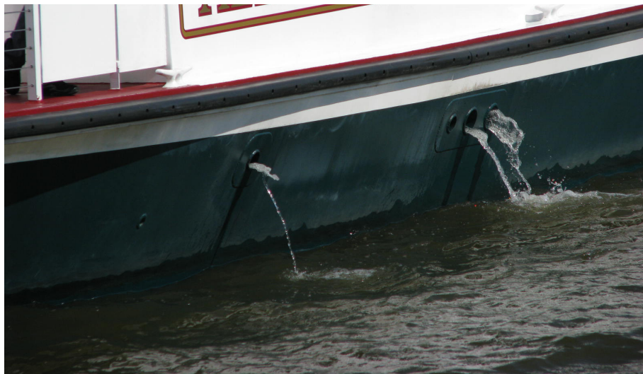
Various Discharges Through Hull Discharge Ports.
