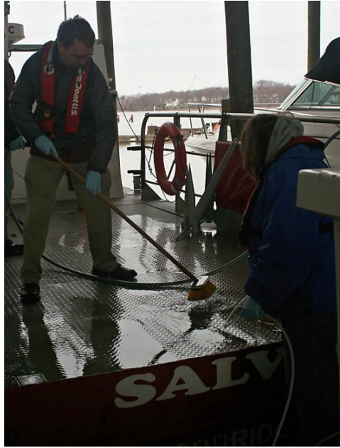
Collecting Deck Washdown Samples from a Tow and Salvage Vessel
