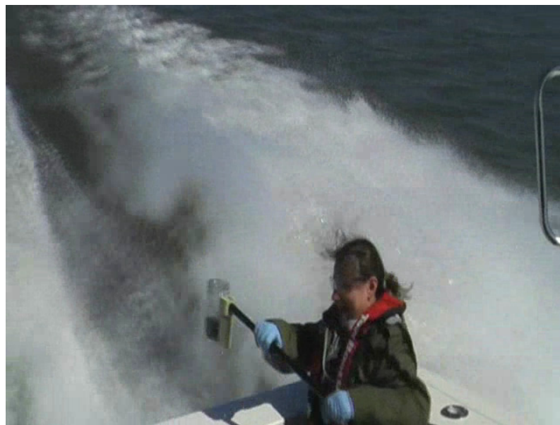
Collecting the Engine Effluent of a Tow and Salvage Vessel at Full Speed
