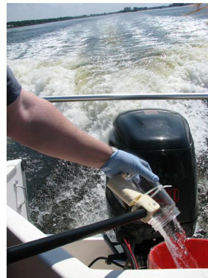
Compositing the Sample in a Lined Bucket.
