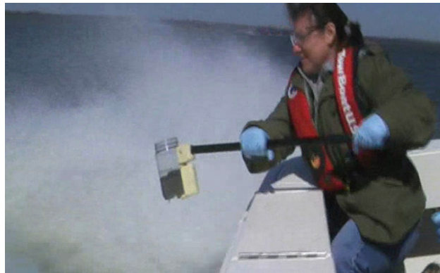
Collecting a Sample of Engine Effluent at Full Speed.
