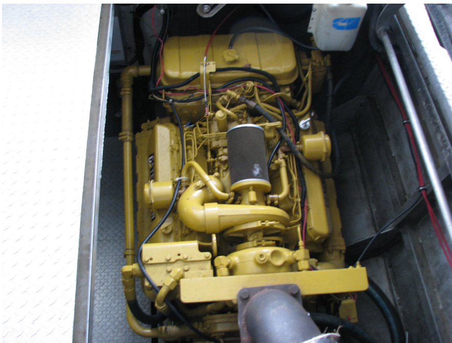
The Inboard Propulsion Engine of a Fire Boat
