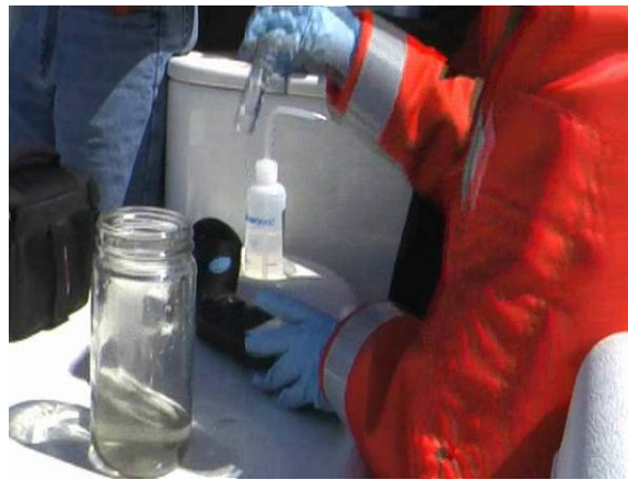
Measuring Total Residual Chlorine Immediately After Sample is Taken.
