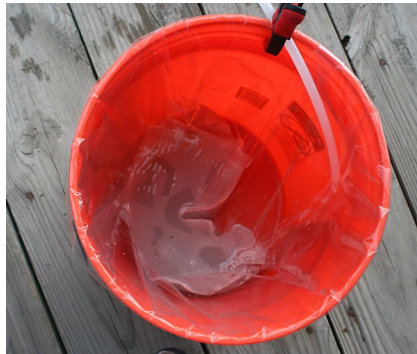
Deck Washdown Sample Collected in a Lined Bucket
