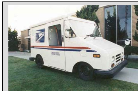
Harbor City, California, 1995 Ten GM Hughes/U.S. Electricar electric LLVs were tested for mail delivery in California and Virginia in the late 1990s.
