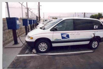
Harbor City, California, 1999 An EPIC charges up at the Harbor City Post Office. EPICs could reportedly go 80 to 90 miles between charges. The vehicles, which letter carriers praised for their quiet, efficient operation, were returned to Daimler-Chrysler in 2001 at the end of their three-year lease.
