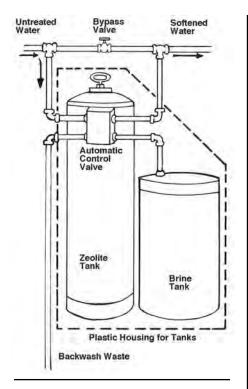
Figure 2. Automatic water softener – two tanks.
