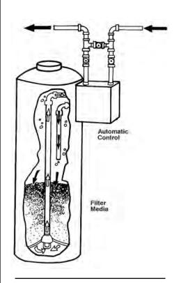
Figure 4. Pressure filter with automatic backwash control.
