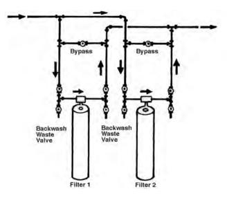
Larger filters are available (16 to 20 inches in diameter), and they provide much better filtration and treatment for higher flows. However, a flow of 20 gpm or more is needed for backwashing (Figure 6).
