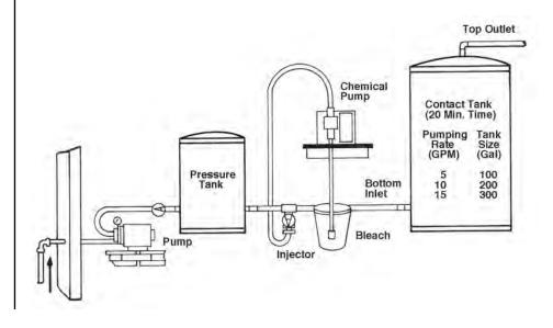
Figure 8. Contact tank size for various pumping rates.
