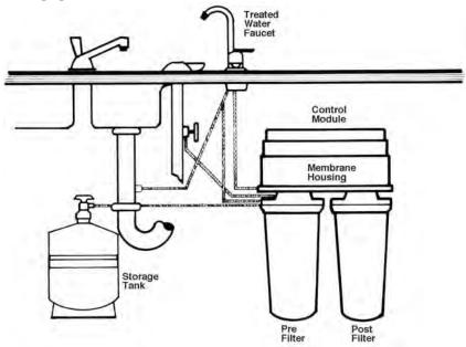
High-capacity RO equipment is expensive, but small-capacity units that can treat about 5 gallons of water per day are available at reasonable prices from equipment dealers. These units are usually located near the kitchen sink and have a two-gallon reservoir to hold treated water for cooking and drinking (Figure 3).
