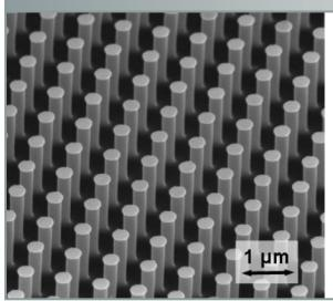
Scanning electron microscope image of a NAPA with a post height of 1000 nm, post diameter of 200 nm, and periodicity of 500 nm
