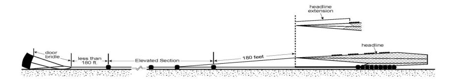
This figure shows the location of elevating devices in the elevated section of modified nonpelagic trawl gear, as specified under § 679.24(f). The top image shows the location of the end elevating devices in the elevated section for gear with net bridles less than 180 feet. The bottom image shows the locations of the beginning elevating devices near the doors and the end elevating devices near the net for gear with net bridles greater than 180 feet.
