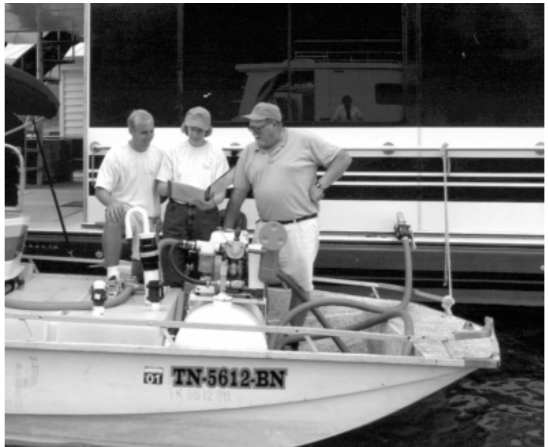
Pump-out boats such as this one on Norris Reservoir are a convenient alternative to fixed-point waste collection systems.
