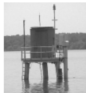
TVA uses a variety of methods to monitor water temperatures in the Tennessee River system, including fixed stations such as the one shown here at Browns Ferry Nuclear Plant.
