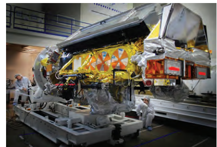
NOAA-N Prime provides a polar-orbiting platform to support environmental monitoring instruments for imaging and measuring the Earth's atmosphere, its surface and cloud cover, including Earth radiation, atmospheric ozone, aerosol distribution, sea surface temperature, and vertical temperature and water profiles in the troposphere and stratosphere. The satellite assists in measuring proton and electron fluxes at orbit altitude, collecting data from remote platforms and is crucial to the Search and Rescue Satellite-Aided Tracking system.
