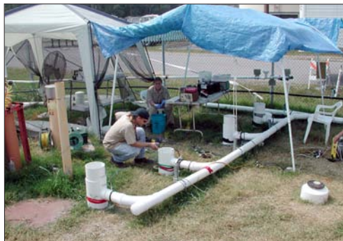
Field tracer injection and monitoring
