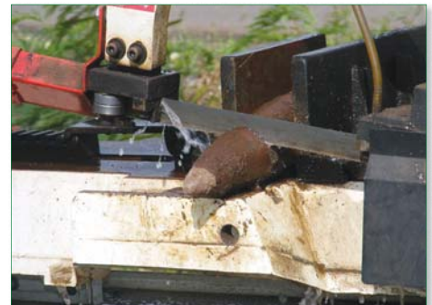
A close-up view of a chop saw used to “demilitarize” a munition shell found at the Molokai landfill. Photo courtesy of ATI, Inc.
