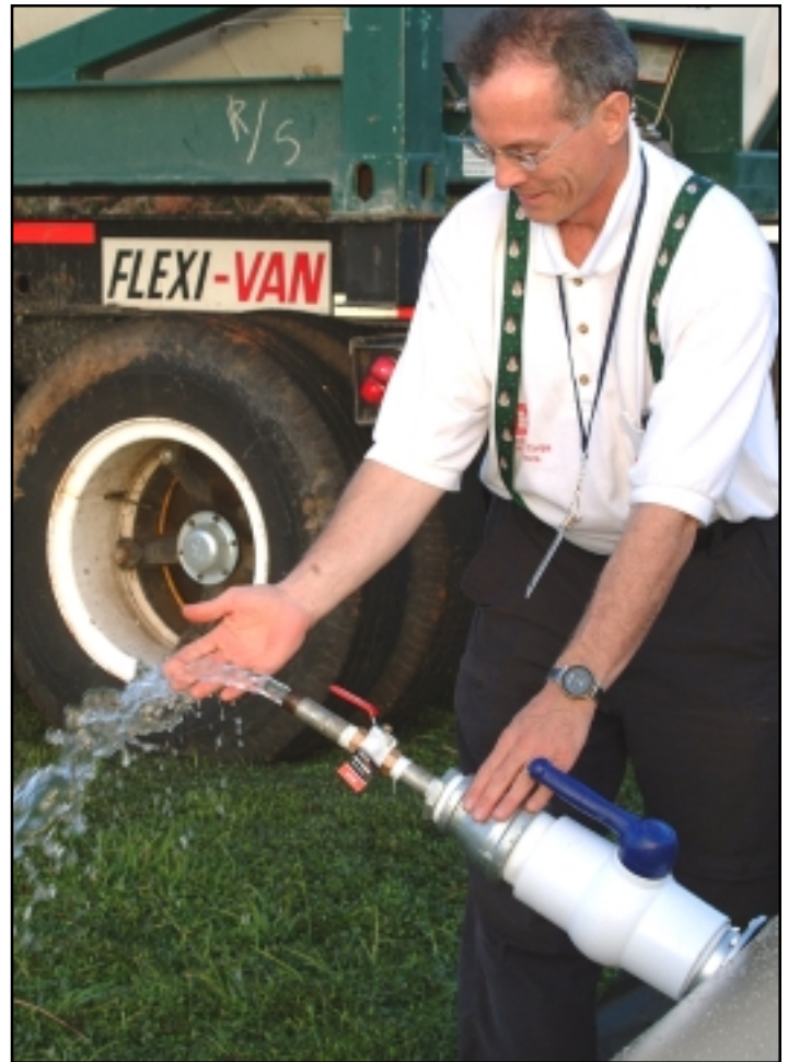
Max Frauenthal, Little Rock District, checks the water pressure on a just-filled 2,642-gallon water bladder that will allow residents to have potable water.
