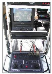
In addition to basic speed, direction and depth controls for the ROV (Remote Operation Vehicle), instrumentation also includes a television, a video cassette tape recorder and a digital recorder for collecting and recording Global Positioning location plots and visual information in both digital and VHS formats.
