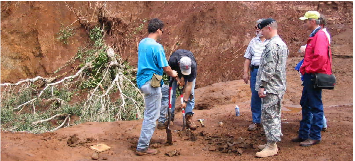
Honolulu District Commander Lt. Col. David E. Anderson observes Honolulu District and State of Hawaii geotechnical engineers collecting soil samples during a dam inspection survey on Kauai. USACE is assisting Hawaii DLNR with inspecting dams on the islands of Hawaii, Maui, Molokai and Oahu. Photo by Maj. Robert Kroning
