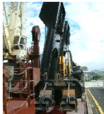
Dragarms on each side of the vessel carry away the sand or silt and deposit it in the hopper bins.
