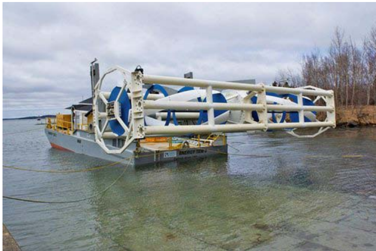
Figure 15. ORPC's Beta Turbine Generator Unit generates clean, renewable electricity by harnessing the energy of the world's rivers and oceans. Photo from Ocean Renewable Power Company, NREL/PIX 17210
