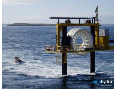
Figure 16. OpenHydro's Open-Center Turbine is designed to be deployed directly on the seabed. The first 6-m test unit produces enough energy to supply 150 average European homes and save the emission of over 450 tons of CO 2 greenhouse gas per year. Photo from OpenHydro, NREL/PIX 17243
