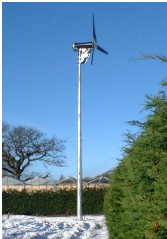
Figure 4. Proven 11 downwind turbine with spring-loaded blade furling design. Photo from Proven Energy
