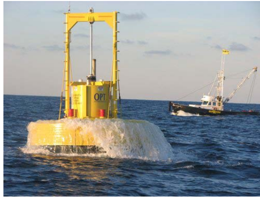
Figure 14. Ocean Power Technologies PowerBuoy wave generation system uses a "smart", ocean-going buoy to capture and convert wave energy into low-cost clean electricity. Photo from Ocean Power Technologies, NREL/PIX 17114
