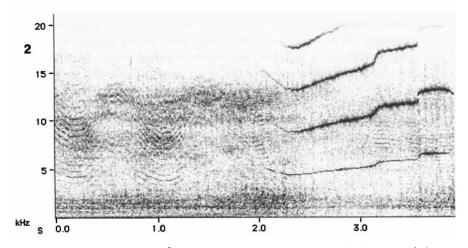
Figure 1. Spectrograms of two sequences containing FM whistles, recorded using a sonobuoy and audio tape recorder. Spectrogram 2 also shows the lower emphases of clicks whose major energy was probably beyond the upper limit of the equipment. The weak, multiharmonic, tonal sounds present at 0.3, 1.0, 2.0, and 3.5 sec in this record probably represent the repetition rate of ultrasonic clicks.
