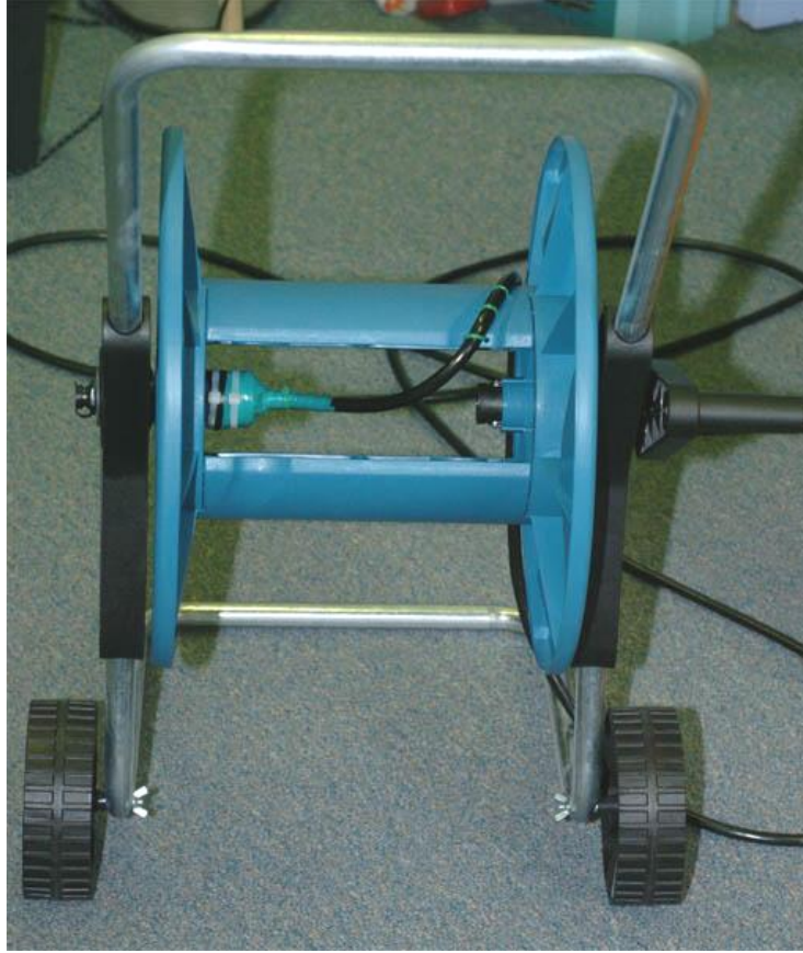
Figure 21. Garden hose reel modified for use as a hydrophone cable reel. Ensure that the hose reel and bolts are made of marine grade stainless steel, or aluminium. An endcap on the connector is important to protect from splashes and allows easy rinsing and cleaning at the end of the day.
