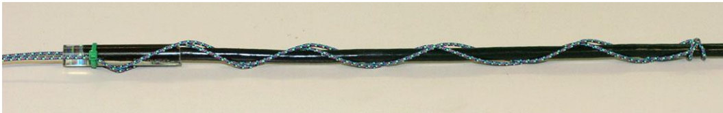
Figure 20. Completed strain-relief weave on the end of a hydrophone cable.
