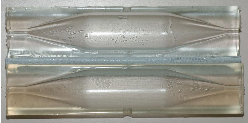
Figure 5. Completed mold after being removed from the PVC form.
