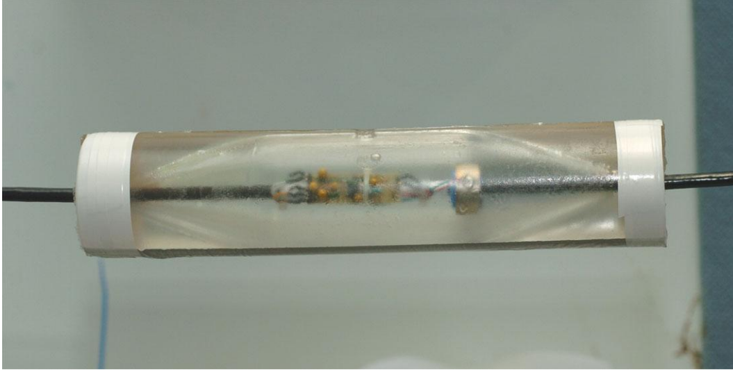
Figure 14. Position of the mold around the pre-amp and hydrophone element prior to casting.
