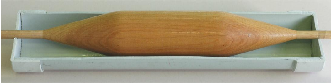
Figure 4. Hydrophone mold making setup. The blank (Fig. 2) is secured within half of the PVC form (Fig. 3).
