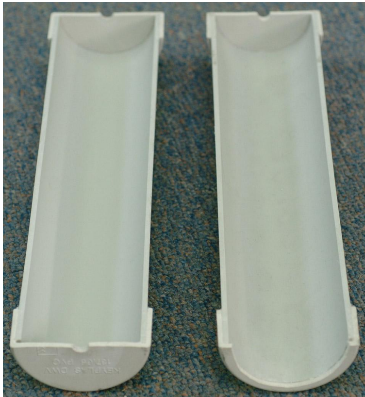
Figure 3. PVC form used for casting the hydrophone mold.
