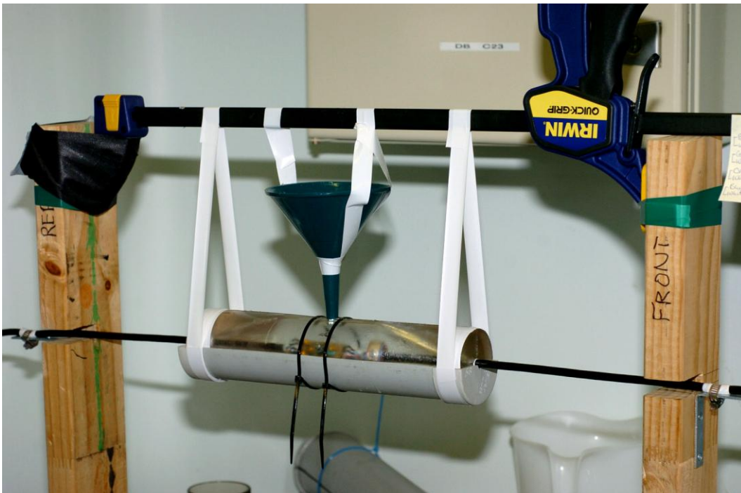
Figure 15. Setup for casting a hydrophone node onto a cable.
