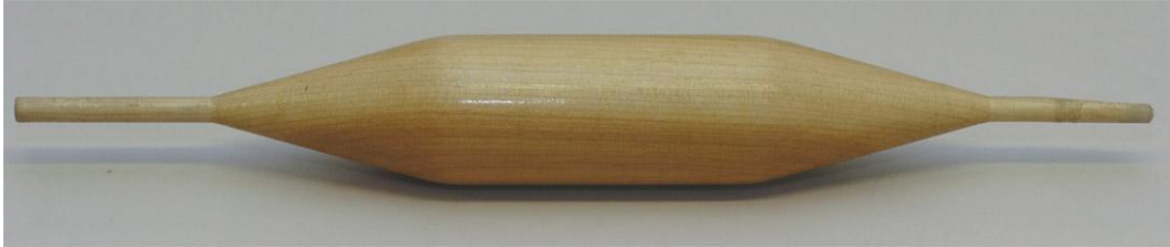
Figure 2. Varnished wooden mold blank used for making a mold for hydrophone casting. The blank is exactly the finished size of the hydrophone and cable.
