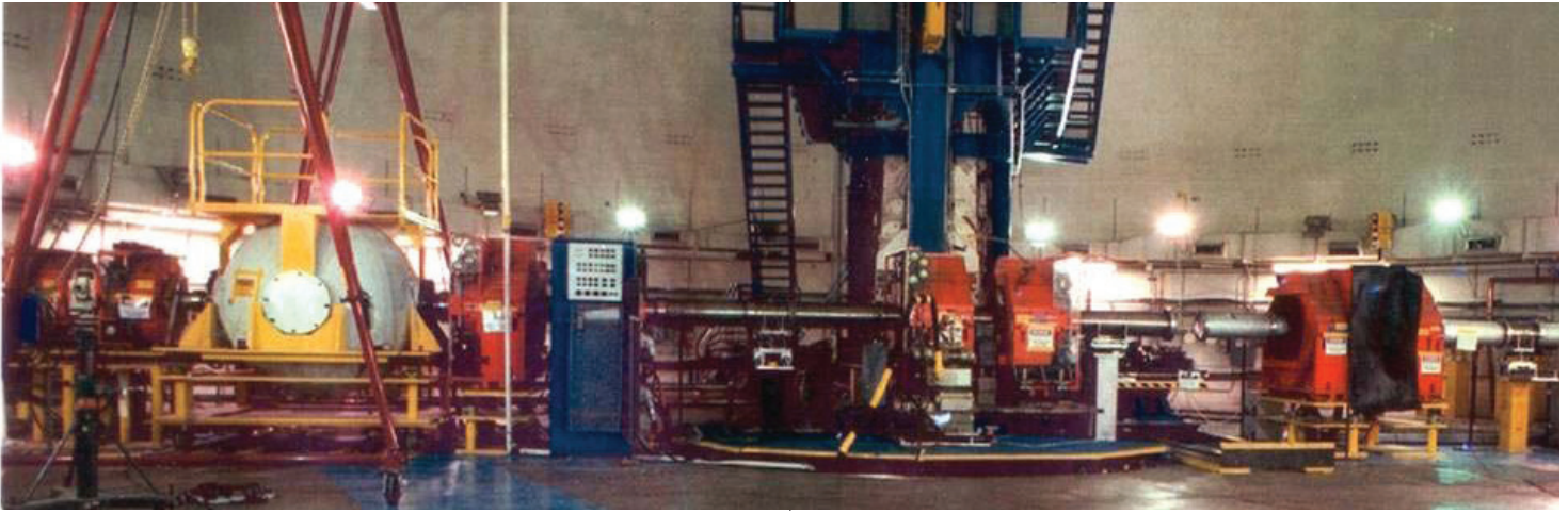
Proton radiography, invented at Los Alamos National Laboratory, employs a high-energy proton beam to image the properties and behavior of materials driven by high explosives.
