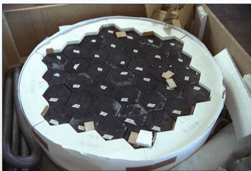
WINDOWED BEAM DOWN AIR RECEIVER
