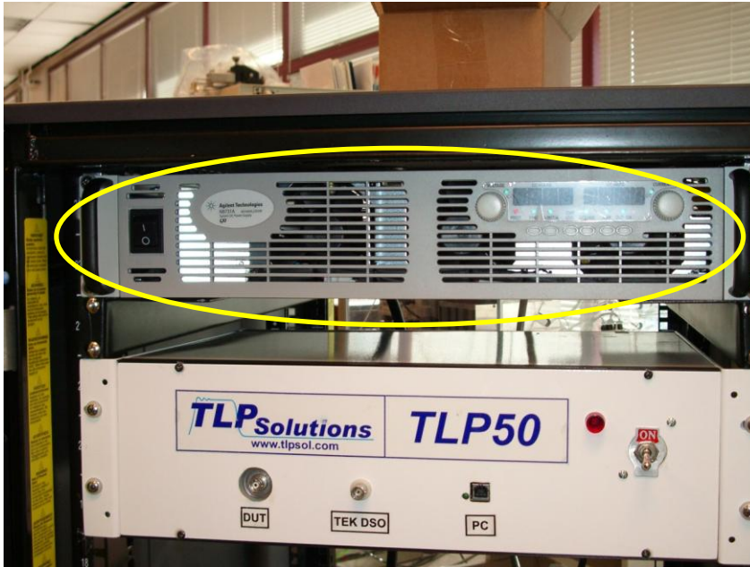
3200 W power supply (400 A, 8 V)
