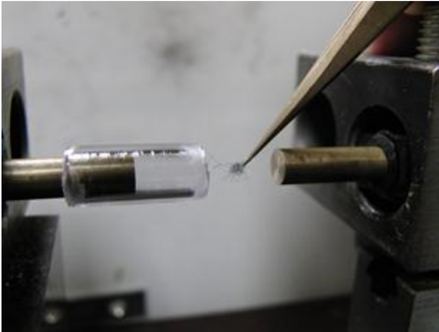
Fine steel wool in tube triggers arc
