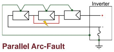
Two failures create new conduction path.
