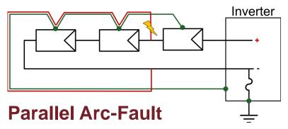
**Two** failures create new conduction path. (Fault current passes through equipment ground but not GFPD) Not Covered in *NEC*
