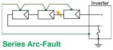
Single failure in intended conduction path.
