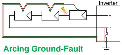
**Single** failure to equipment ground. (Fault current passes through GFPD)
