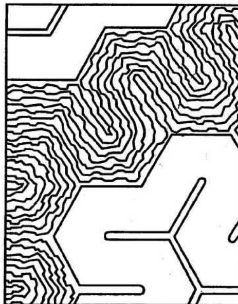
MEANDER MODEL (PECHOLD, 1968) CHAINS HAVE QUASI-PARALLEL PACKING
