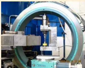
Residual Stress and Texture (REST) diffractometer at NFL Studsvik
