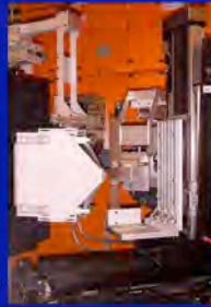
Welded cruciform specimen mounted on NRSF2 for stress mapping.
