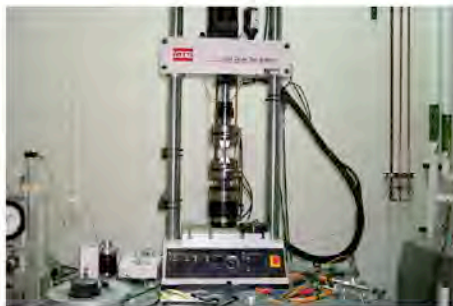
Axial and torsional test system (MTS 858 AT)
