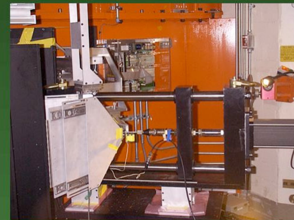
A tensile specimen mounted on load frame on NRSF2.
