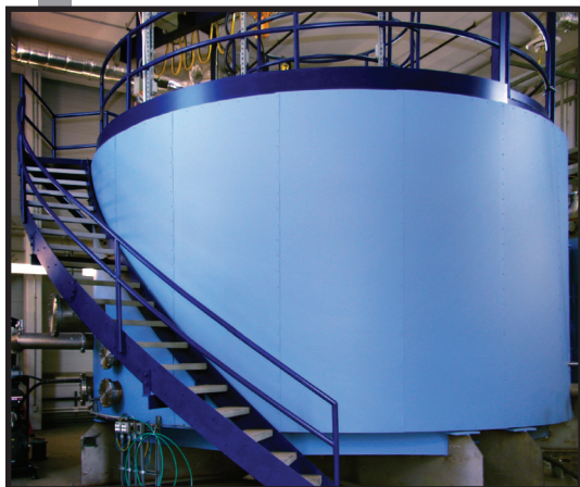
Evacuated final flight path of the backscattering spectrometer.
