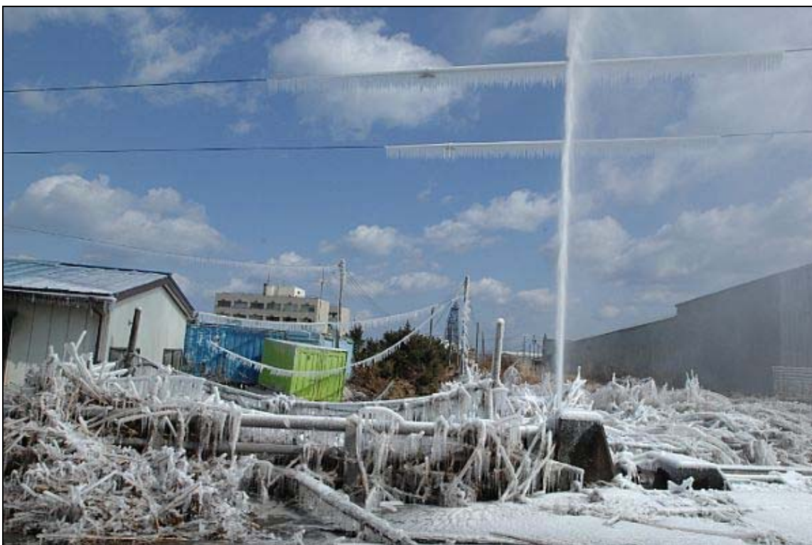
Figure 3.A Damaged Water Pipe Shoots into the Air, Hachinohe, Japan
