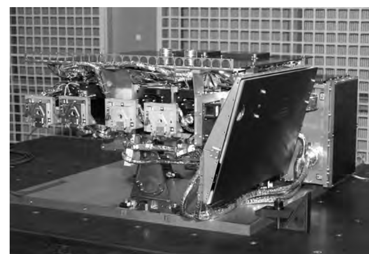
This is the completed EVE instrument. It will have the highest time resolution (10 seconds) and the highest spectral resolution (better than 0.1 nm) ever achieved by a space-based solar observatory.
