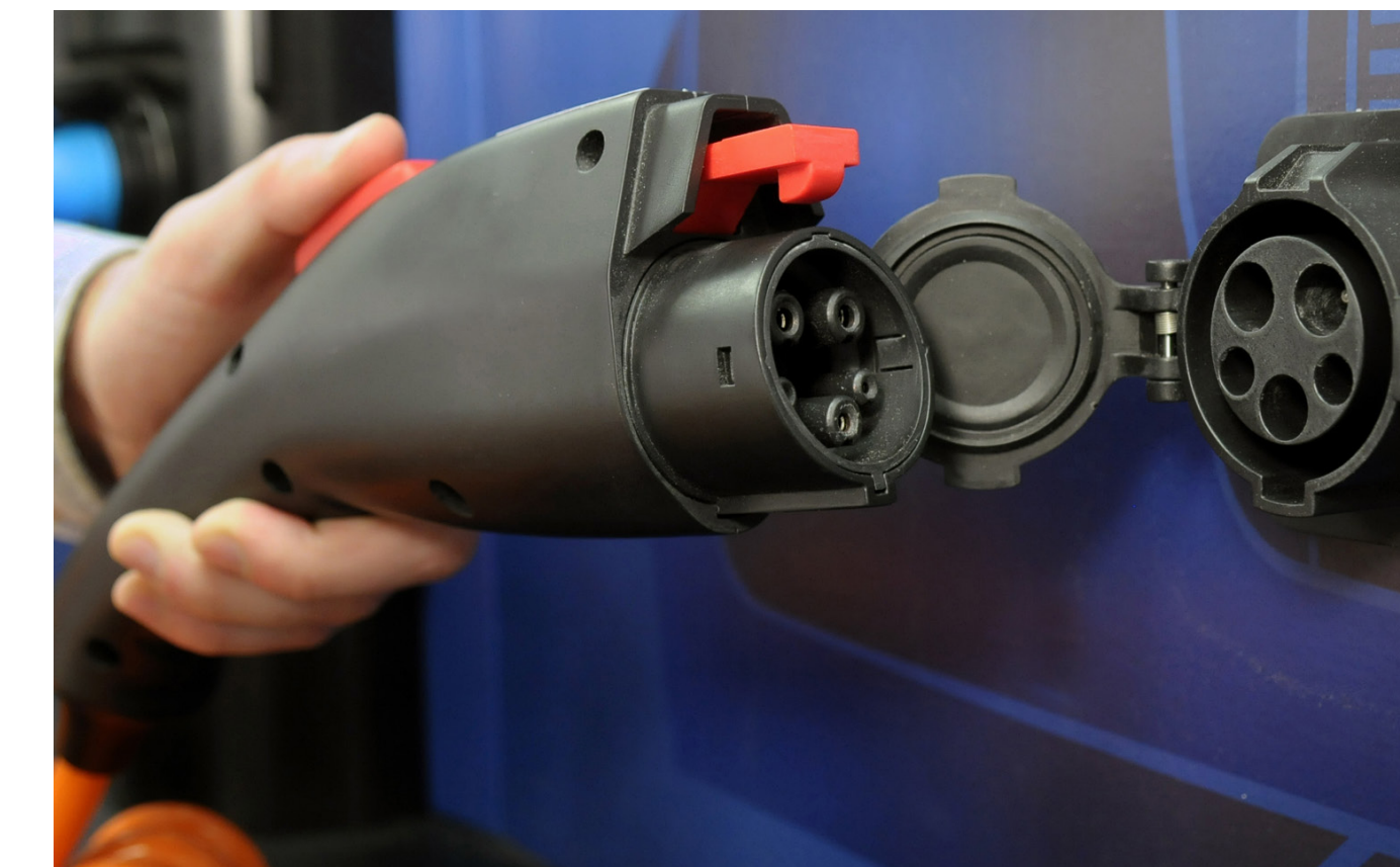
Argonne helped to develop the standard for a uniform plug-in vehicle connector that facilitates both charging and communication.
