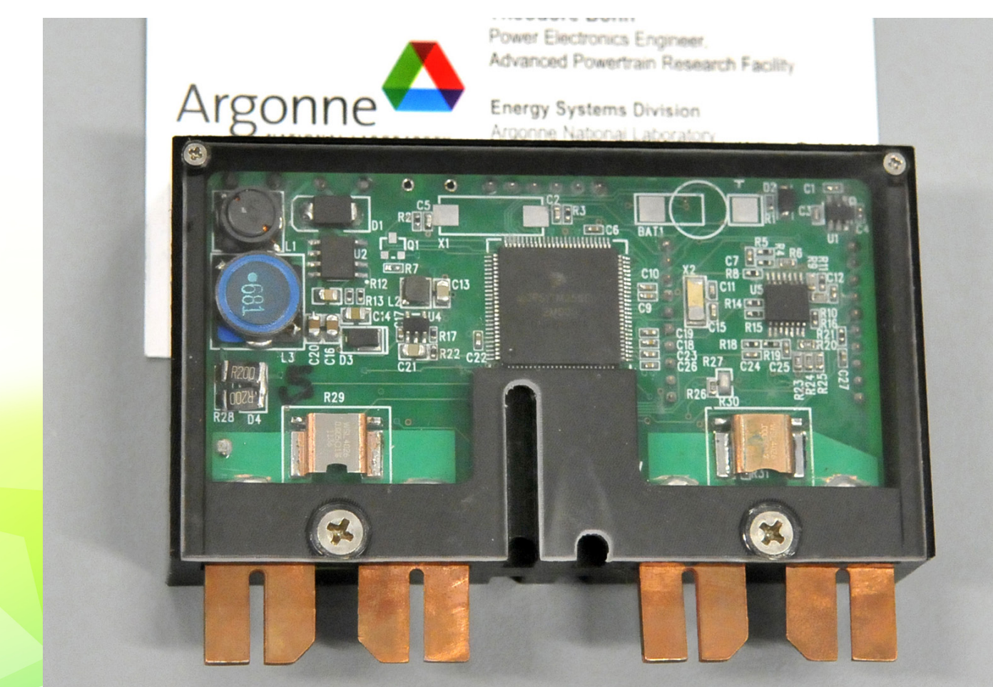
A prototype of Argonne's compact metrology system. These systems are end-use measurement devices (EUMD) that measure and communicate energy usage information to ensure accurate consumption readings and fair billing.
