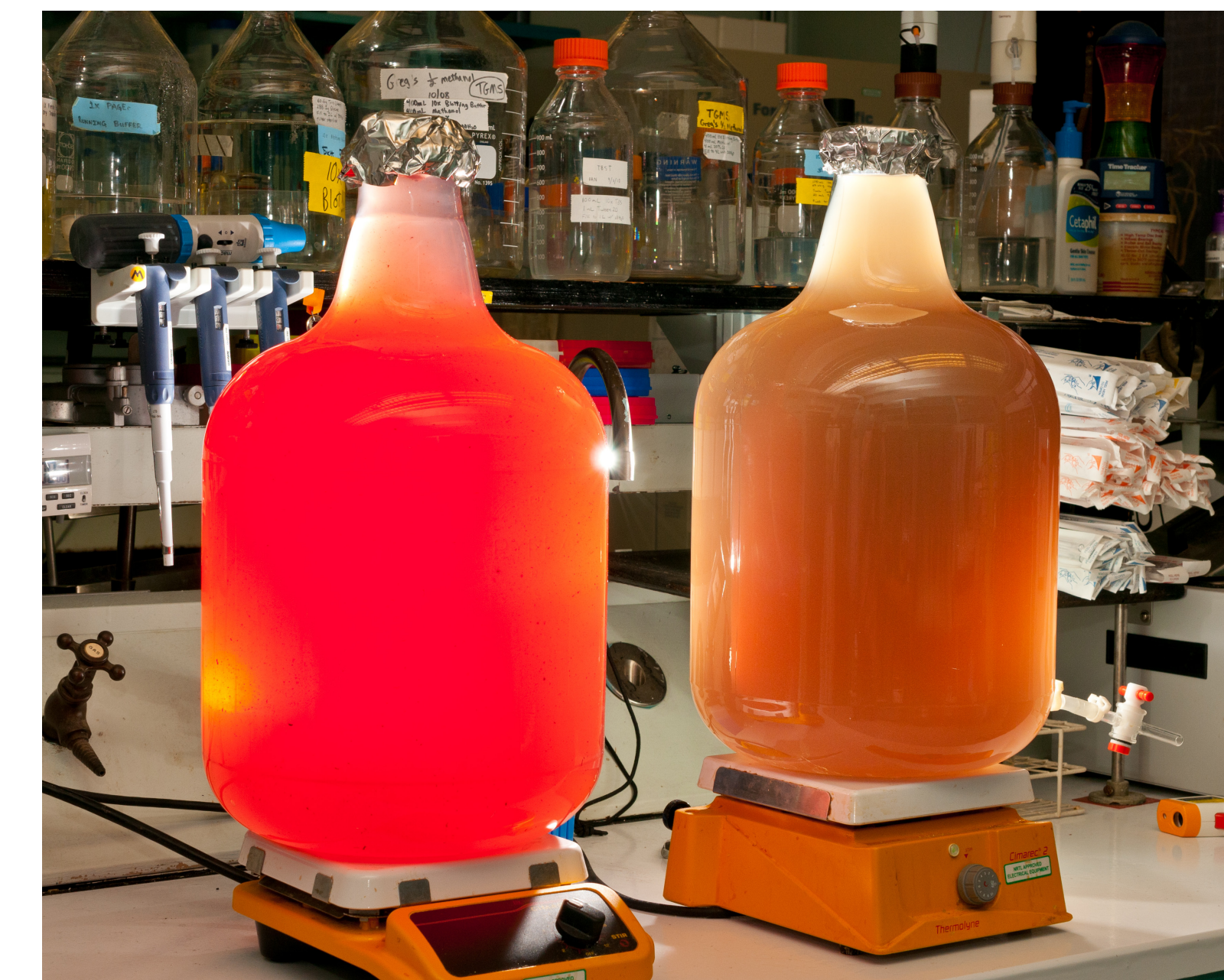
The photosynthetic bacteria within the EBR efficiently convert waste from kitchens or latrines into long-chain alcohols. Once separated from the fermentation broth, these serve as surrogates for diesel fuel that can be used alone or in blends to power vehicles or generators.
