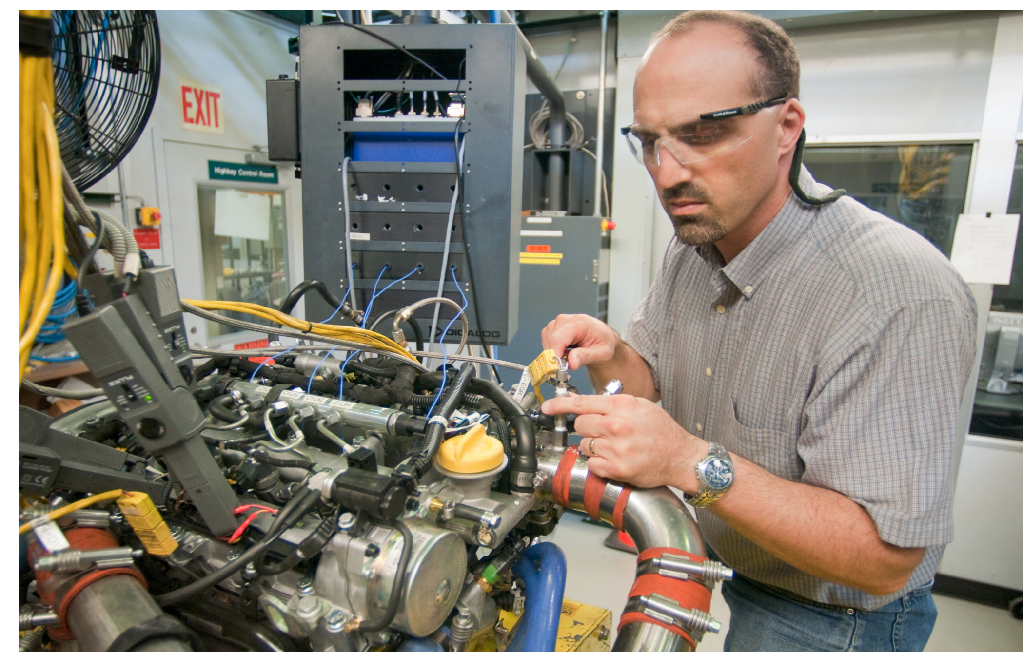
Argonne engineer Steve Ciatti inspects diagnostic instruments to insure proper operation of the low-temperature combustion engine.
