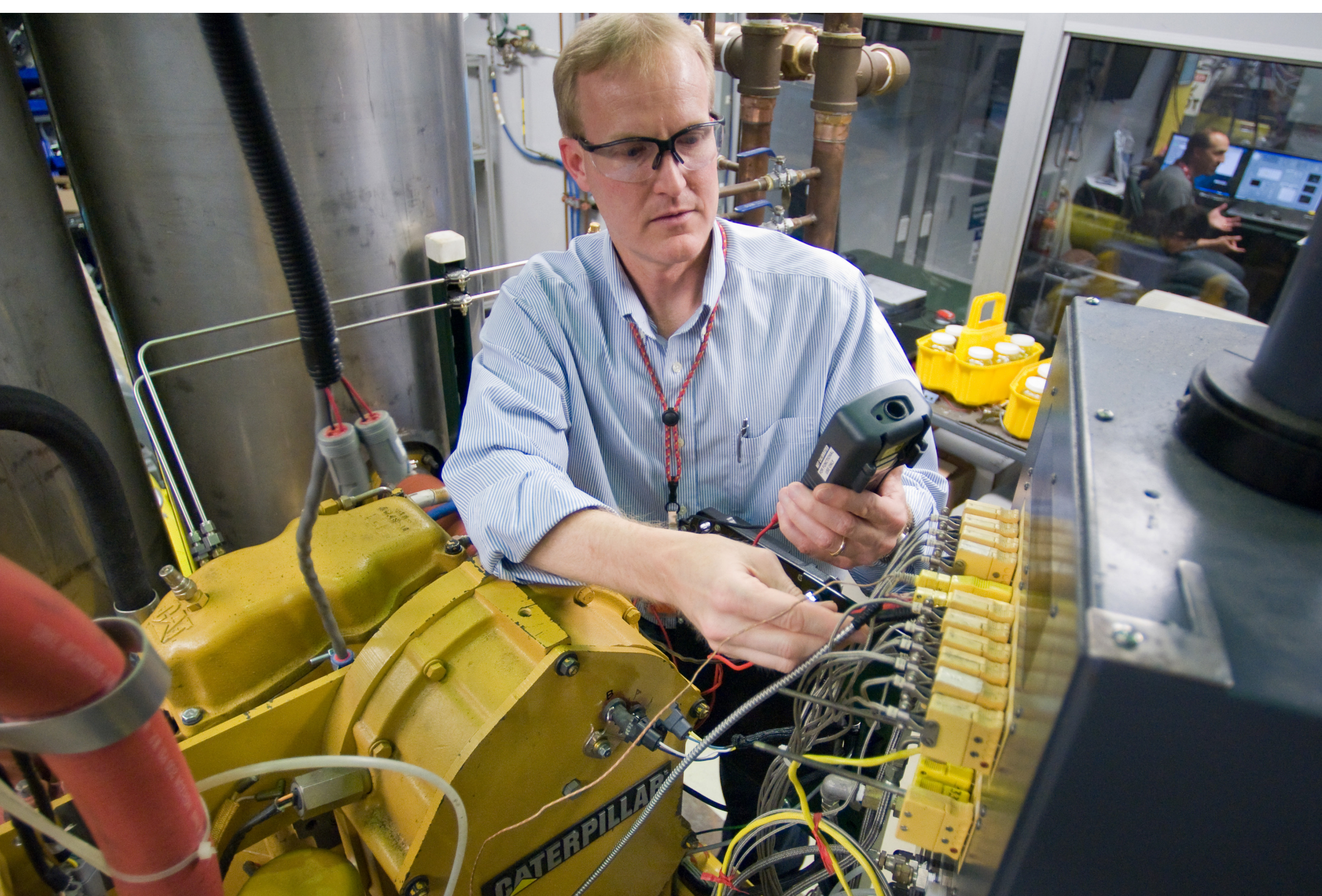
Argonne mechanical engineer Doug Longman uses the laboratory's engine testing facilities to evaluate the performance and emissions of newly developed biofuels.
