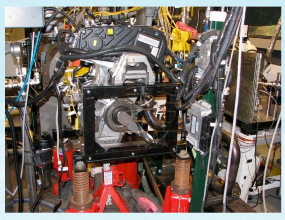
Argonne's experimental setup includes a GM 1.9 L, 110 kW @ 4500 rpm (designed to run on #2 diesel), and a Bosch II generation common rail injection system.
