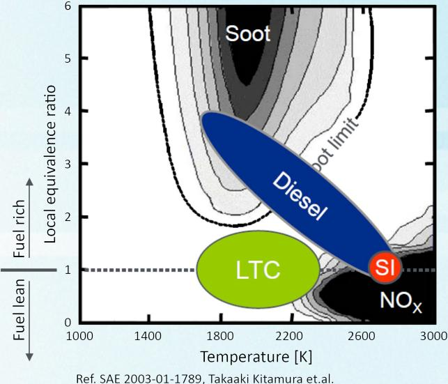
This chart illustrates how LTC avoids both soot and NO<sub>x</sub> by controlling fuel/air mixing (equivalence ratio) and by slowing down the rates of reaction (peak combustion temperature).
