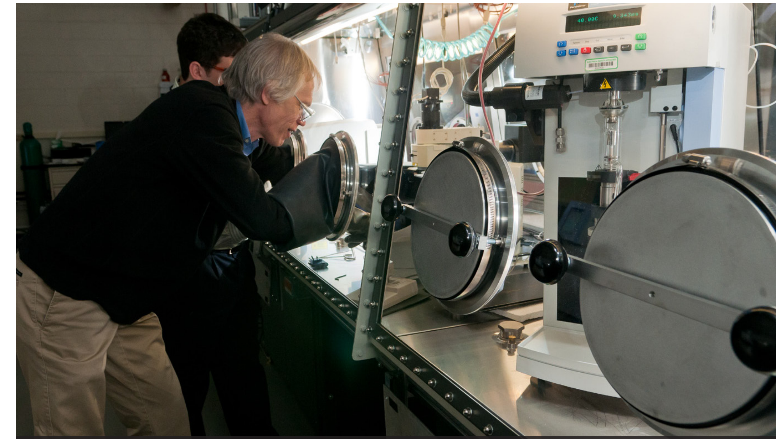
Two Argonne scientists prepare a sample for characterization to answer the question of what changes occurred during the life of a battery.
