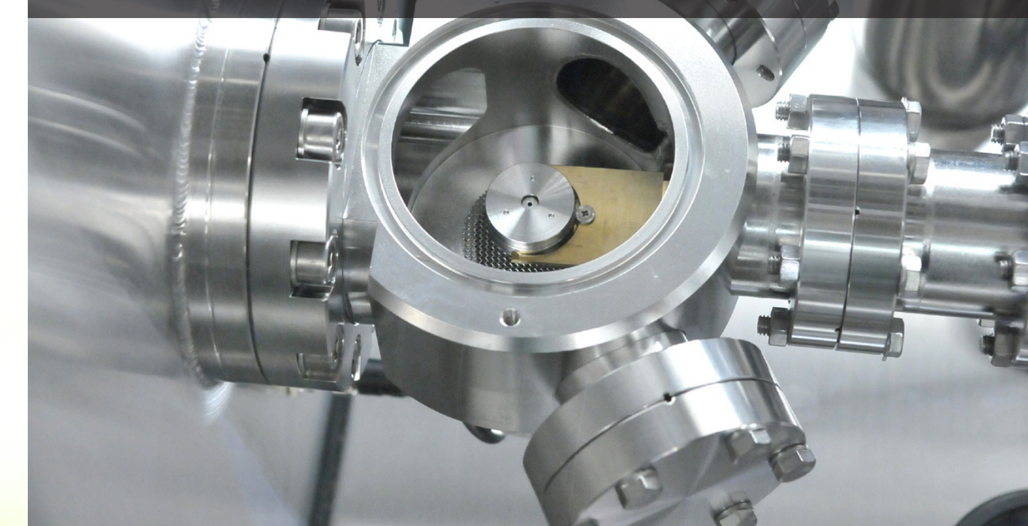
Peering into another world, a sample is mounted in the XPS for characterization of the nature of what on the surface of a material.
