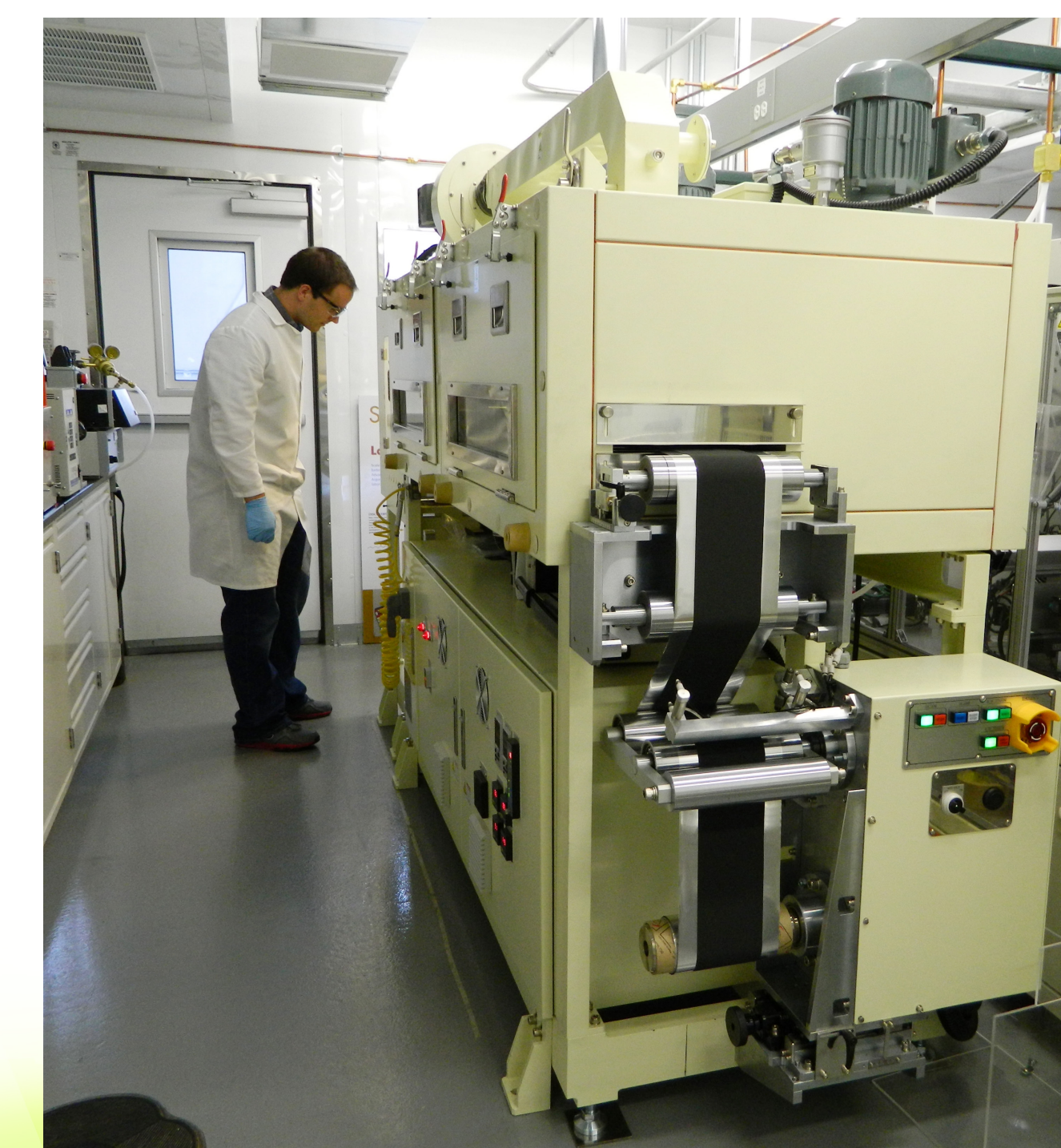
Argonne engineering assistant Steve Trask operates a state-of-the-art electrode coating system to make the positive electrode used in prototype lithium-ion cells.
