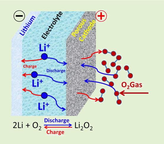
Argonne's ultimate goal is to transfer battery innovations to the marketplace, providing industry with processes, materials, performance testing data and finished cells. And what lies beyond the lithium-ion battery? Argonne is constantly working on new battery chemistries and materials. Take the futuristic lithium-air battery: it uses air as fuel and offers up to 10 times the energy density of lithium-ion.
