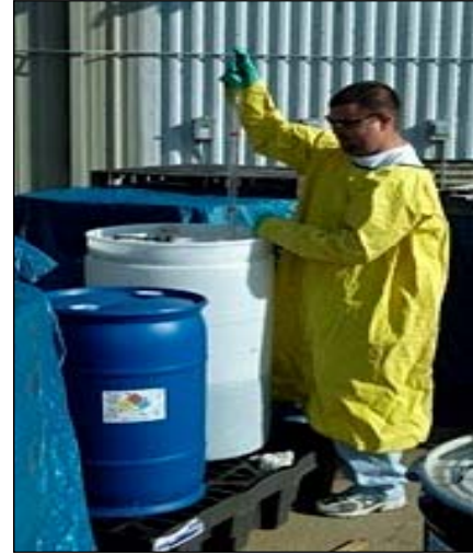
Secondary Containment in Use
