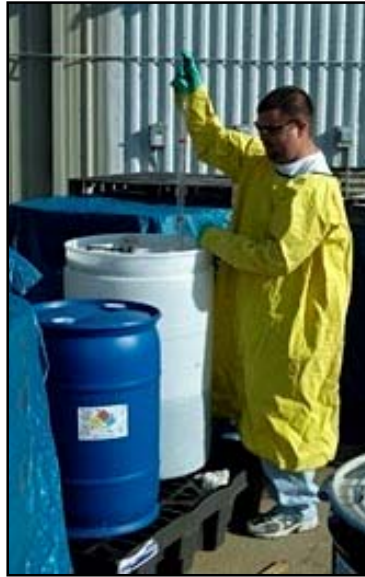
Secondary Containment in Use
