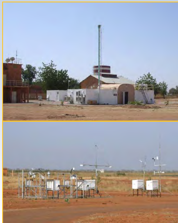
Located near the airport in Niamey, the ARM Mobile Facility obtained measurements from January through December 2006, spanning both the wet and dry seasons. These data are allowing scientists to study radiative feedback of the Earth's atmosphere in the region, including the interaction of local clouds and the West African monsoon with dust and aerosols.
