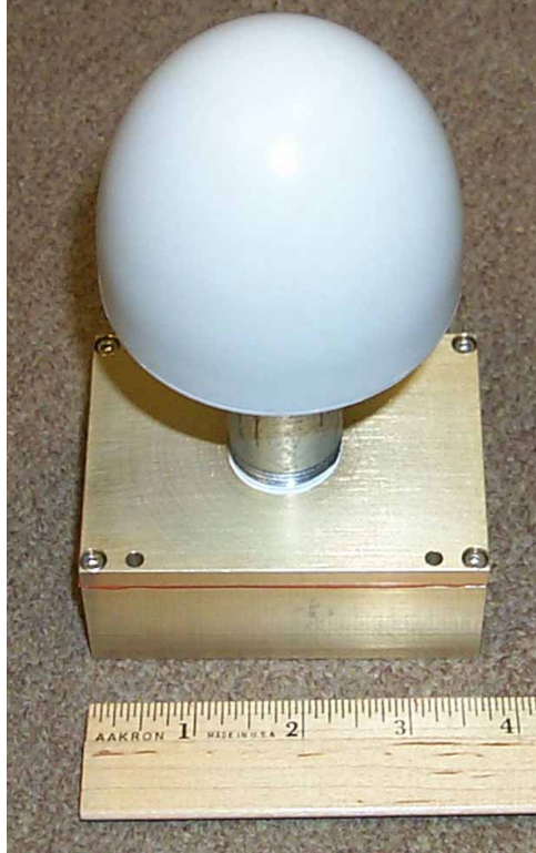
Figure 2-11. GPS Receiver/Antenna Configuration.
